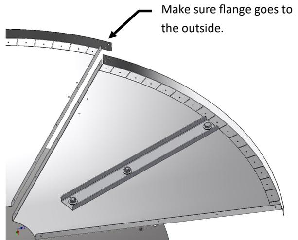
Note: Some air seals and hubs are provided with more mounting holes than may be required. This is done intentionally to make the air seals more interchangeable between units.
