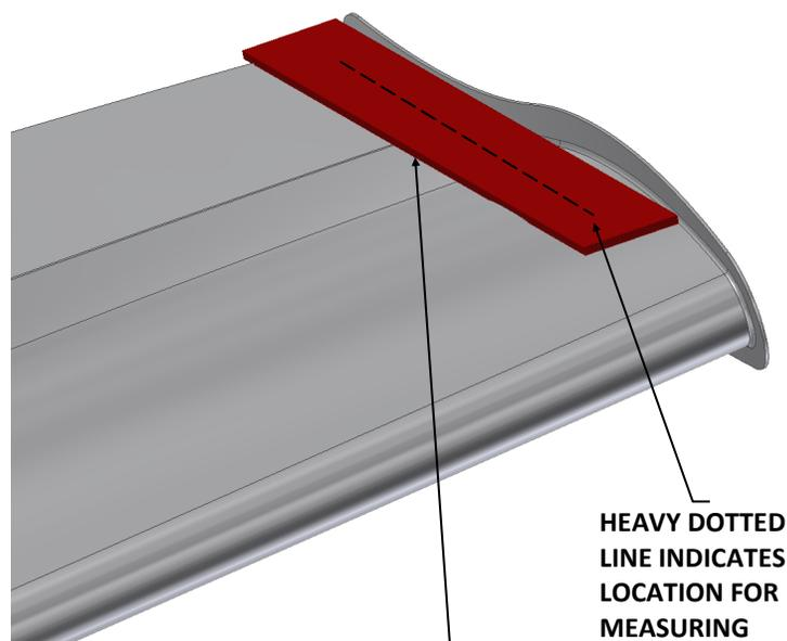
HEAVY DOTTED LINE INDICATES LOCATION FOR MEASURING BLADE ANGLE
