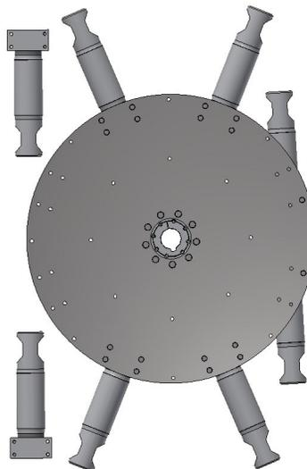
The hub requires rod ends / blocks installed.
