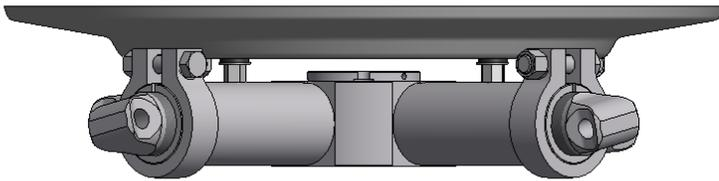
Air Seal Installed on Hub, Bushing on top.
