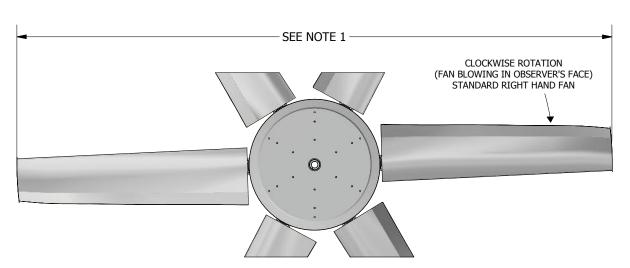
NOTE 1: MAXIMUM FAN DIAMETER (BLADES HORIZONTAL - AS SHIPPED) EQUALS NOMINAL FAN DIAMETER. ADJUSTMENT OF  $\pm 1.5$  INCHES POSSIBLE AT INSTALLATION.
