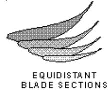
1. The individual blades will be narrow at the tip, where the blade velocity is high, and will widen toward the hub, where more blade area is required due to lower blade velocity.
